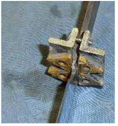
So go to the grinder, run the belt to the edge of the platen and grind away as shown. The belt won't cut the carbide (true even for ceramic belts). Make the plunge cut on one side, then flip the blade over and repeat on the other. That was EASY.
